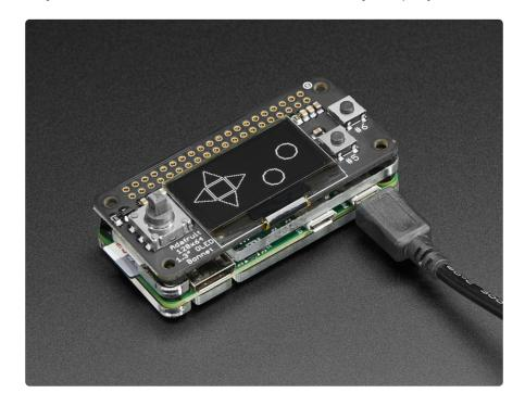
These displays are small, only about 1.3" diagonal, but very readable due to the high contrast of an OLED display. This screen is made of 128x64 individual white OLED
