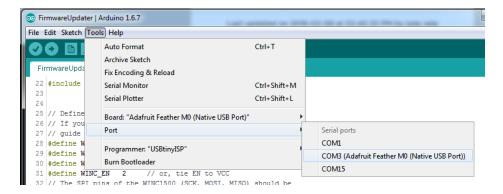
Upload it to your Feather. Make sure the Serial console is not open before or after uploading.
