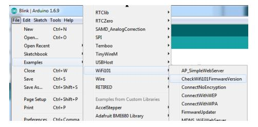
Upload to your Arduino and open up the Serial Console at 9600 baud:
