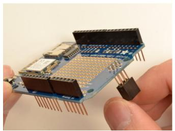
Insert the 2x3 stacking header as shown.
