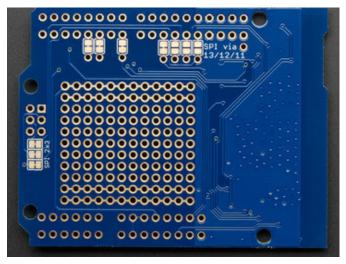
If you happen to want to use 11/12/13 rather than the SPI header, turn the board over, you can cut the 3 jumpers next to the 2-3 ISP header and solder the open jumpers between the SPI pins and D11/12/13
