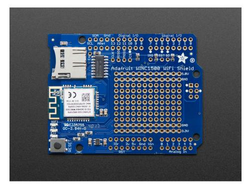
The Adafruit ATWINC1500 WiFi Shield uses SPI to communicate plus some GPIO for control, so with about 6 wires, you can get your wired up and ready to go. Right now the Atmel-supplied library works best with SAMD21-based
