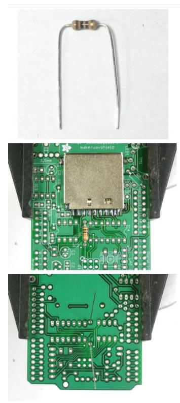
Next, we will solder all of the many resistors. The 10K resistor **R6** is first.
