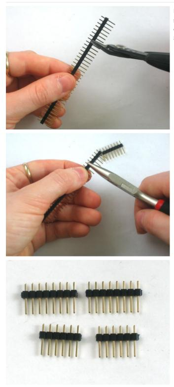
Next, break the 36-pin header strip into smaller sections so that the shield can be placed on the Arduino. You can use pliers or diagonal cutters. Clip off 2-6pin and 2-8pin pieces.
