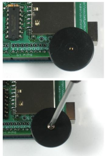
Next you can install the thumbwheel. Use a #0 screwdriver. Align the thumbwheel so it 'grabs' the potentiometer, then gently screw it in place.
