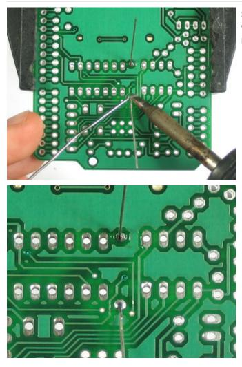
Solder the leads to the pads (metal ring) by heating both with the side-tip of the iron for 3 seconds and then poking in a bit of solder.
