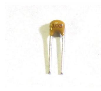
Next is the 0.01uF ceramic capacitor **C8**. The tricky part here is that in older kits there are many 0.1uF ceramic capacitors in the kit that look identical to the 0.01uF!
