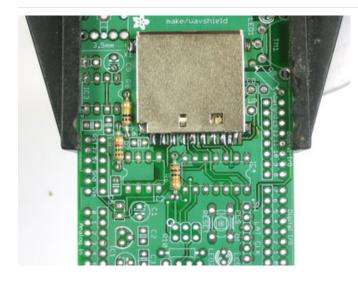
Finish up the resistors by placing  $\ensuremath{\text{R8}}$  (100Kohm), and  $\ensuremath{\text{R7}}$  (1.5K)
