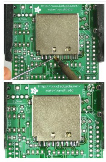
Now go thru and solder the 8 leftmost pins that stick out from the holder. The three rightmost pins are thinner and closer together so they are tougher to solder. Luckily they are not used and you simply skip them (although the photo shows them done).
