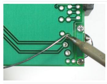
Solder all 5 pins of the potentiometer. Use plenty of solder so that it has a lot of mechanical strength.
