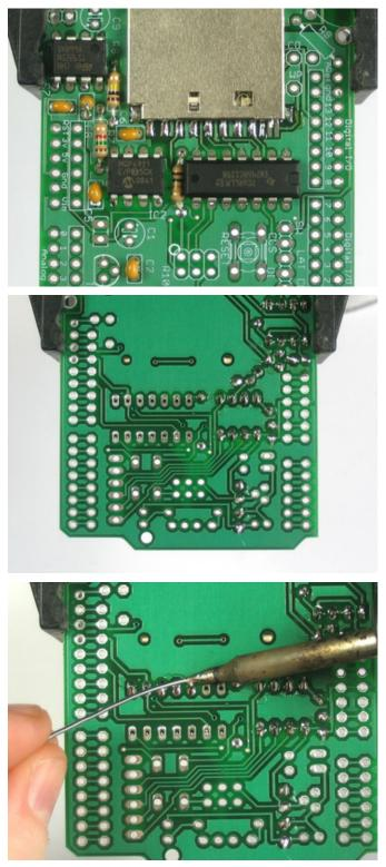
Next is **IC4**, the buffer to talk to the SD card. Match up the notch just like you did with the smaller chips.
