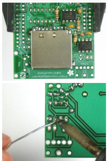
Next is the operational-amplifier (op-amp) **IC3**. It is used to buffer and amplify the output, so that it can drive a small speaker or headphones.
