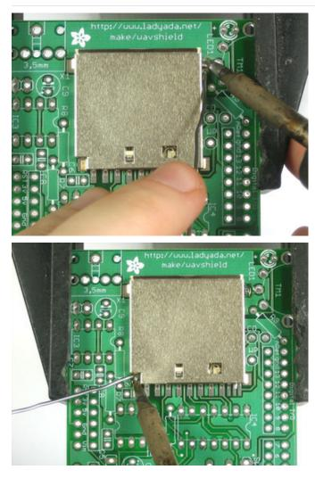
We'll start with the four side tabs that are used to mechanically secure the card holder in place.
