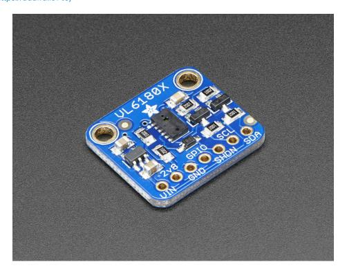
This is the 'little sister' of the VL53L0X ToF sensor, and can handle about 5mm to 200mm of range distance. It also includes a lux sensor. If you need a larger range, check out the VL53L0X which can measure 50 - 1200 mm.
