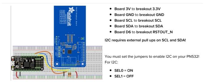
Here's an example of wiring a Feather M0 to the breakout with I2C:
