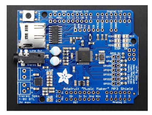
There's a lot of stuff going on in this shield! Lets look at the board and all the pinouts. The amplifier version and nonamplifier version both use the same PCB so the pinouts are the same. We'll talk about just the amplifier separately at the bottom
