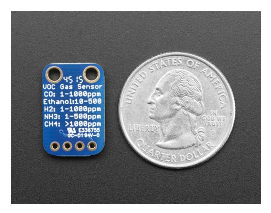
Using it is easy: Power it with 5 VDC and read the analog voltage off of the output pin. When gasses are detected, the analog voltage will increase in proportion of detected gas. When powered, the heater draws about 25-35mA. You can use the EN pin to power it off (pull it high to 5V to turn off) to conserve energy. Just make sure to wait a second after turning the heater on to make sure its all heated before taking readings.
