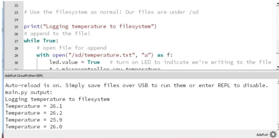
The screenshot shows the Adafruit CircuitPython REPL interface. The top pane displays Python code for logging temperature to an SD card. The bottom pane shows the output of the program, including the message 'Logging temperature to filesystem' and four temperature readings: 26.1, 26.2, 25.9, and 26.0.
