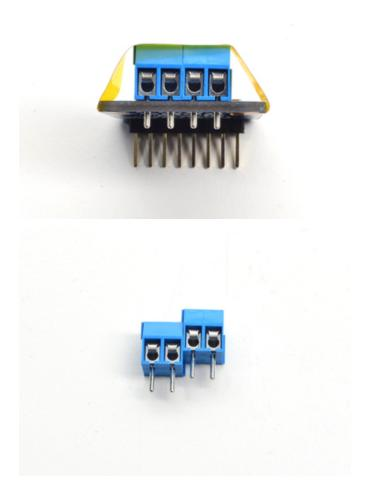
Solder in both pins of each terminal block. You can remove the tape when done.
