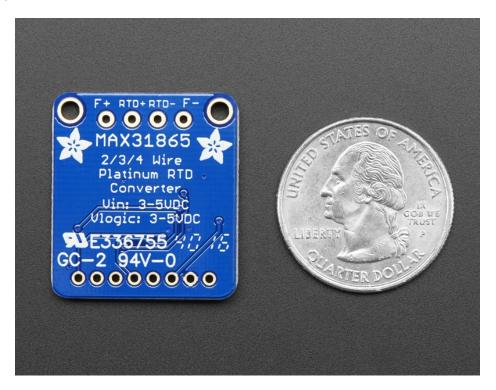
We've carried various MAXIM thermocouple amplifiers and they're great - but thermocouples don't have the best accuracy or precision, for when the readings must be as good as can be. The MAX31865 handles all of your RTD needs, and can even compensate 3 or 4 wire RTDs for better accuracy. Connect to it with any microcontroller over SPI and read out the resistance ratio from the internal ADC. We put a 0.1% resistor as a reference resistor on the breakout.
