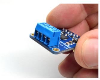
Next we will solder in the two 3.5mm terminal blocks used to connect power & the motor to the breakout board.
