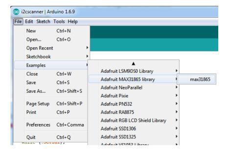
Upload to your Arduino and open up the serial console at 115200 baud to see a print out of the sensors data. The MAX31865 doesn't actually return the resistance it measures. Instead it returns the *ratio* between the resistance measured and the **Rref** reference resistor.
