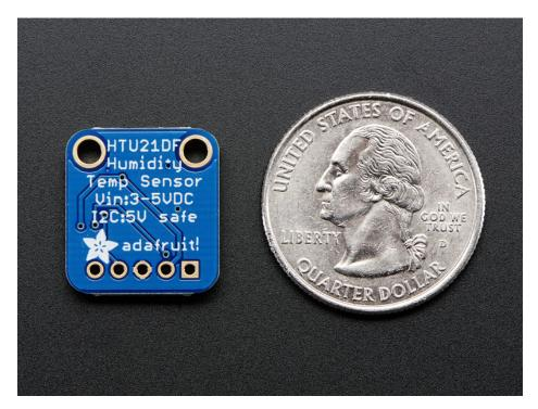
This I2C digital humidity sensor is an accurate and intelligent alternative to the much simpler Humidity and Temperature Sensor - SHT15 Breakout (http://adafru.it/1638) It has a typical accuracy of ±2% with an operating range that's optimized from 5% to 95% RH. Operation outside this range is still possible - just the accuracy might drop a bit.
