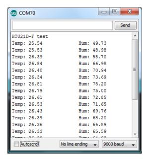
You can try breathing on the sensor to increase the humidity. The sensor reacts very fast!
