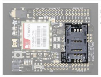
The SIM card holder it on the right side of the shield. It holds a very-standard "Mini SIM" Micro SIMs will not work! Make sure you get a "Mini SIM"
