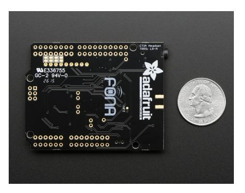
Each order comes with one tested and assembled FONA shield and a stick of 0.1" male header.**Required Arduino, SIM** card, battery, antenna and other accessories are not included! Some light soldering is required to put the headers onto the shield. You can also grab some stacking headers if you would like to stack a shield on top (https://adafru.it/dsu)
