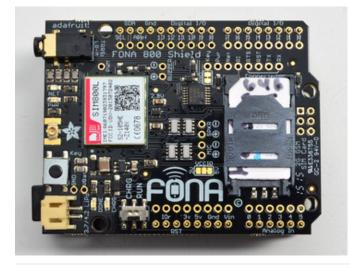
The SIM should be secure and flat in the holder
