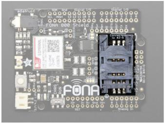
The SIM card holder it on the right side of the shield. It holds a very-standard "Mini SIM"
