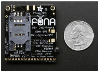
The SIM card holder is on the back. It holds a verystandard "Mini SIM"
