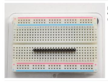
Prepare the header strip: Cut the strip to length if necessary. It will be easier to solder if you insert it into a breadboard - **long pins down**
