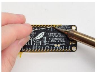
Flip & Tack Solder After flipping over, solder one or two points on each strip, to 'tack' the header in place
