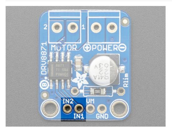
These are the inputs to the motor control. IN2 goes to OUT2, IN1 goes to IN1. Use up to 5.5V DC logic on these pins. You can PWM the inputs up to 200KHz, but lower frequencies will be more efficient.
