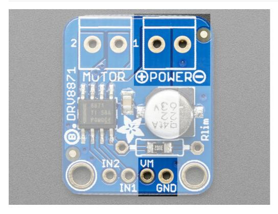
These two sets of pads are connected internally so you can use breadboard or terminal blocks to provide motor
