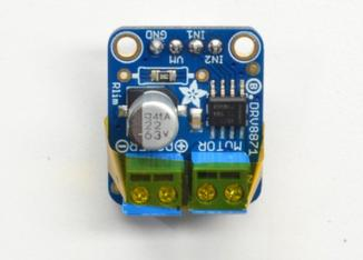
Solder in both pins of each terminal block. You can remove the tape when done.
