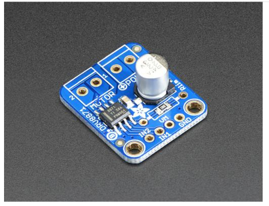
Crank up your robotics with powerful **Adafruit DRV8871** motor driver breakout board. This motor driver has a lot of great specs that make it useful for a wide variety of mechatronics. In particular, the simple resistor-set current limiting and auto-magic PWM support make it super easy to use with almost any brushed DC motor.
