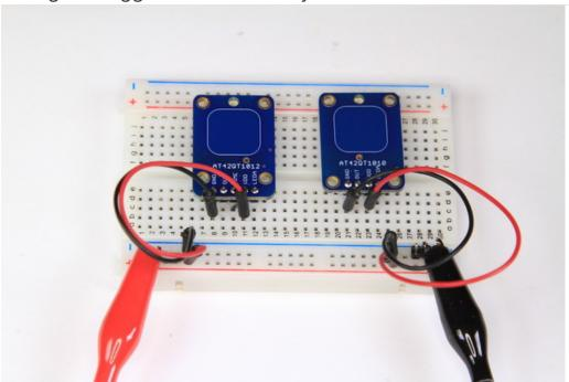
These two breakouts are very similar and can be powered by anything from 1.8V to 5.5V DC. Simply connect Ground to GND and the positive voltage to VDD. The standalone sensors are fully functional without further connections.
