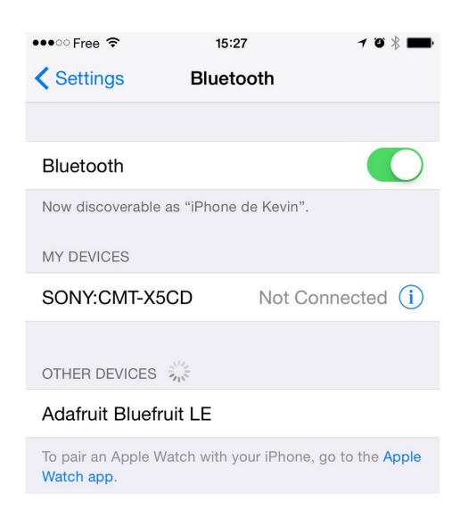
Once the bonding process is complete the device will be moved to the **MY DEVICES** category, and you can start to use the Bluefruit LE module as a keyboard:
