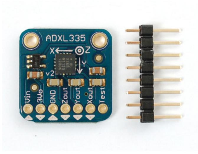
The **ADXL335** can measure at least +/- 3G in the X, Y and Z axis. It is perfect for high-resolution static acceleration measurements such as tilt-sensing, as well as for moderate dynamic accelerations from motion, shock or vibration.
