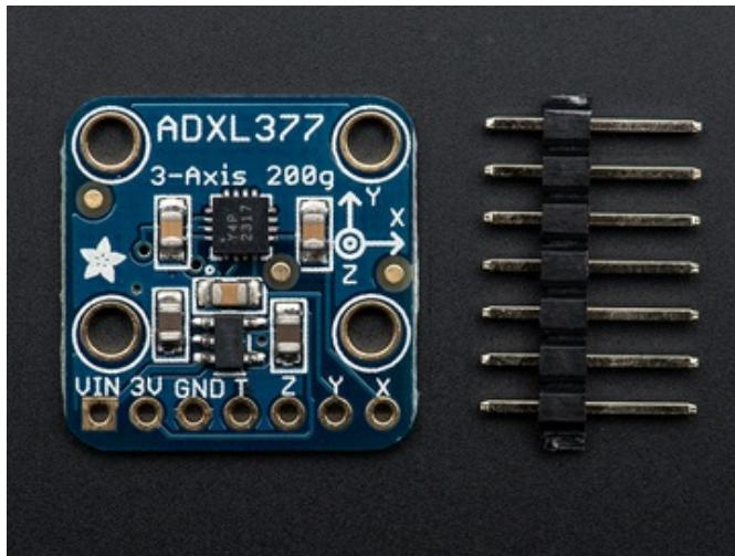
The **ADXL377** can measure at least +/- 200G(!) in the X, Y and Z axis. This is the sensor for measuring extreme dynamic accelerations encountered in applications such as rocketry experiments and high-impact shock measurements.
