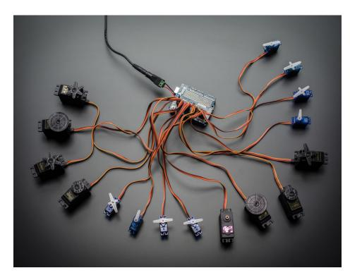
Driving servo motors with the Arduino Servo library is pretty easy, but each one consumes a precious pin - not to mention some Arduino processing power. The Adafruit 16-Channel 12-bit PWM/Servo Driver Shield will drive up to 16 servos over I2C with only 2 pins. The on-board PWM controller will drive all 16 channels simultaneously with no additional Arduino processing overhead. What's more, you can stack up to 62 of them to control even more servos - all with the same 2 pins!
