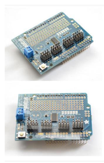
Place the 2 pin terminal block so it faces out. Also place the 3x4 headers so the short pins are plugged into the shield and the long pins are sticking up
