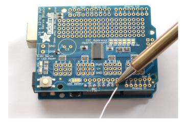
Solder each of the pins to secure the shield to the headers
