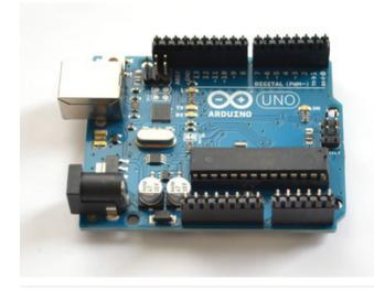
Break apart the 0.1" header into 6, 8 and/or 10-pin long pieces and slip the long ends into the headers of your Arduino
