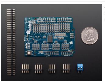
Check you have everything you need: assembled shield PCB, 0.1" male header, 4 of 3x4 male header, and a 2 pin terminal block
