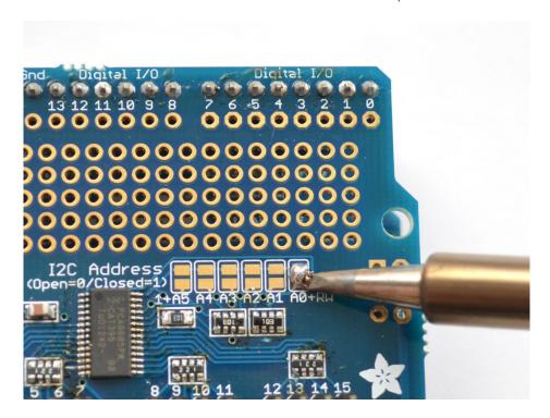
Board 0: Address = 0x40 Offset = binary 00000 (no jumpers required)
