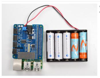
Or, for portable use, a 4 or 5 x AA battery pack can be connected to the terminal block.
