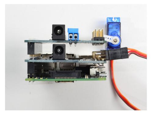
Even though HATs are not intended to be stacked, you can stack up to 62 HATs and not have an address collision, for up to 992 PWM outputs! You'll still need to provide power and write code for all those outputs but they can all share the same SDA/SCL pins no problem.
