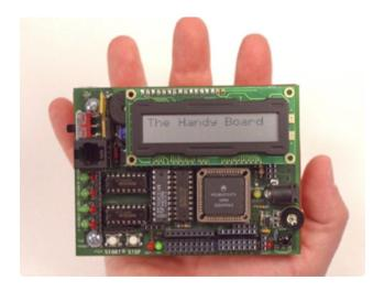
The brains of the 6.270 robot was this robotic control board called the Handy Board. Perhaps because it was handy and fit into your hand? Anyhow it looked like this. All through hole parts with a 16x2 LCD.
