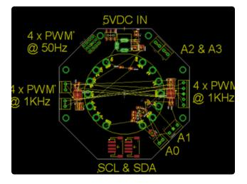
I also started sketching out the PCB design. Just to see what would fit! I decided on the power supply (5V) and how the Circuit Playground would attach.
