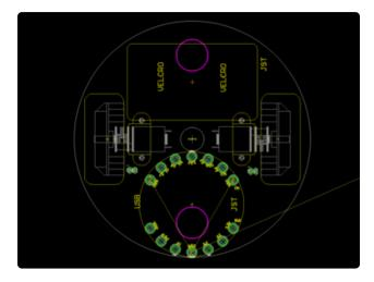
The "CPX Bot" would have the Circuit Playground bolt onto the body and control two micro DC motors. On the opposite side, a velcro'd on battery box would provide power. The motor control circuitry and sensors would be on the PCB itself.
