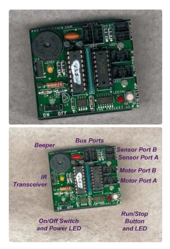
What I find fascinating is how close the Handy Cricket was to an "Arduino of Robotics" but many years before Arduino was invented!
