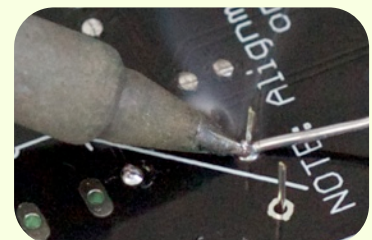
Solder and trim the excess.
