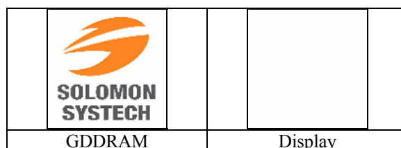
Figure 10-8 : Example of Entire Display ON
