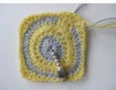
Combination of tilt sensing and potentiometer using regular wool and conductive wool from Schoeller.
