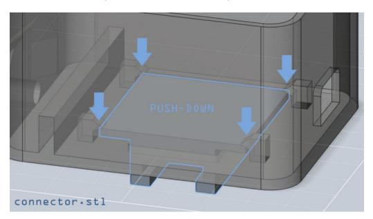
Insert the **connector.stl** part inside the enclosure, through the bottom opening with the flat end facing up. Apply pressure to the corners of the connector to snap them into place.
