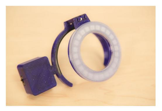
Close up the enclosure by snapping the lid on and slide the switch on to power up the ring! The clip snaps onto most DLSR camera lenses such as the 100mm or 24-70mm prime lenses.
