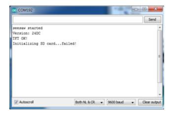
The sketch waits until the serial port is opened (you can make it auto-start once you know things are working by removing the while (!Serial); line
