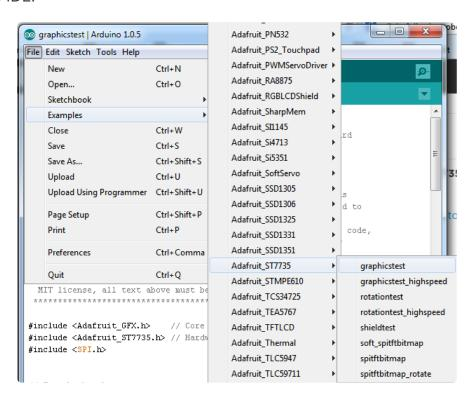
After restarting the Arduino software, you should see a new **example** folder called **Adafruit\_ST7735** and inside, an example called **graphicstest**.
