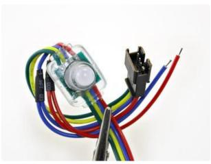
Your pixels will have one end with a receptacle - these tend to be the input side on flat shaped pixels but we've found that isn't true 100% of the time so don't rely on this as a way of determine which end is the input
