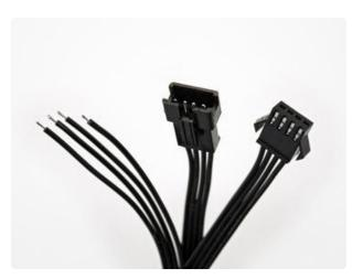
Mating connectors for both are available in the Adafruit shop. These have a housing at one end and four tinned wires at the opposite end...the wires can be soldered directly to your circuit, or strip a little more insulation to press these into Arduino pin sockets.
