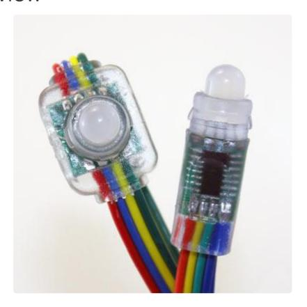
RGB Pixels are digitally-controllable lights you can set to any color, or animate. Each pixel contains an RGB LED and a controller chip molded into a 'dot' of silicone, with flanges so they can be pushed into holes in thin sheet material. The dots are waterproof and rugged — they're typically used to make outdoor signs.
