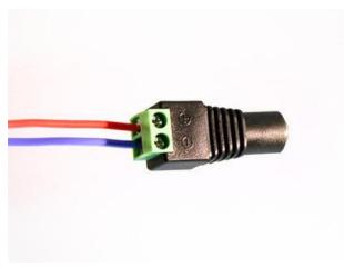
The female DC power adapter (http://adafru.it/368) mates with either of the above power supplies. Screw terminals clamp down on the power leads at the end of an LED strand, so there's no soldering required.
