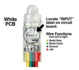
For older bullet pixels with a white circuit board inside, look for the "INPUT" label printed on the board. With this side facing you, the set of wires in front are the input — data arrives here — and the wires underneath are the output to the next pixel.
