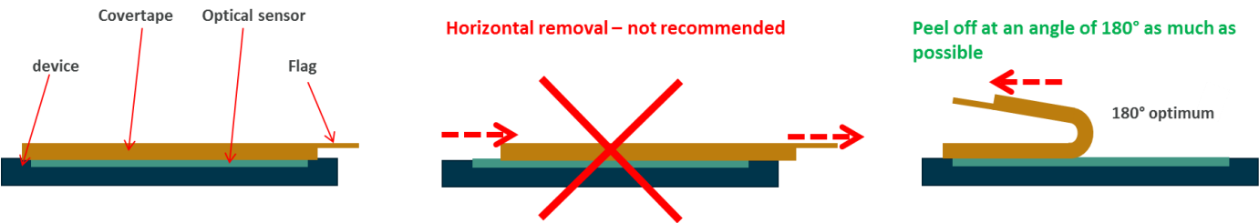
Figure 2: Grab the flag of the covertape and peel it off in an angle of 180° as much as possible.
