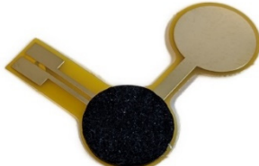
SEN0028 with NANOCOMP-CRC-10X10 material
