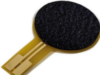
SEN0017 with NANOCOMP-CRC-15X15 material
