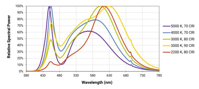
The following graph is the result of a series of pulsed measurements at 1400 mA and  $T_J$  = 85 °C.
