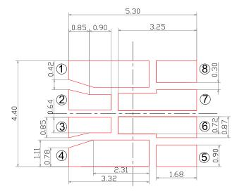
• Tolerance of measurement of the dimension is ±0.1.
