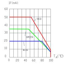
MAXIMUM FORWARD DC CURRENT VS, AMBIENT TEMPERATURE.
