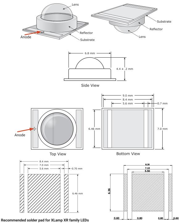
Recommended stencil pattern for XLamp XR family LEDs (hatched area is opening)
