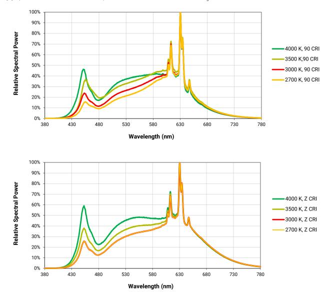
The following graphs are the result of a series of pulsed measurements at 800 mA and  $T_1$  = 85 °C.
