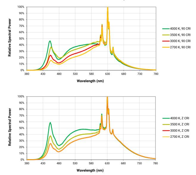
The following graphs are the result of a series of pulsed measurements at 720 mA and T<sub>1</sub> = 85 °C.
