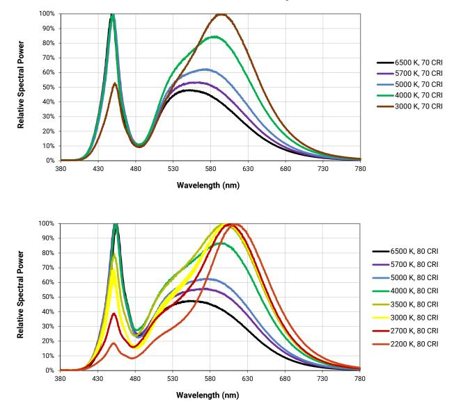
The following graphs are the result of a series of pulsed measurements at 550 mA and T<sub>1</sub> = 85 °C.
