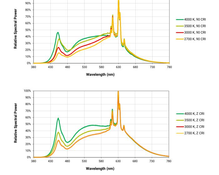
The following graphs are the result of a series of pulsed measurements at 1100 mA and  $T_1$  = 85 °C.
