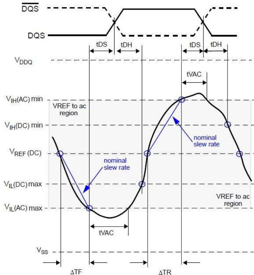
$$\text{Setup Slew Rate} = \frac{V_{REF}(DC) - V_{IL}(AC)\max}{\Delta TF}$$
