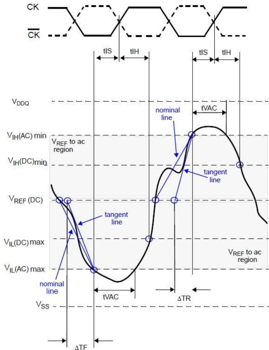
$$\text{Setup Slew Rate} = \frac{\text{tangent line} [ V_{REF}(DC) - V_{IL}(AC)\max ]}{\Delta TF}$$
