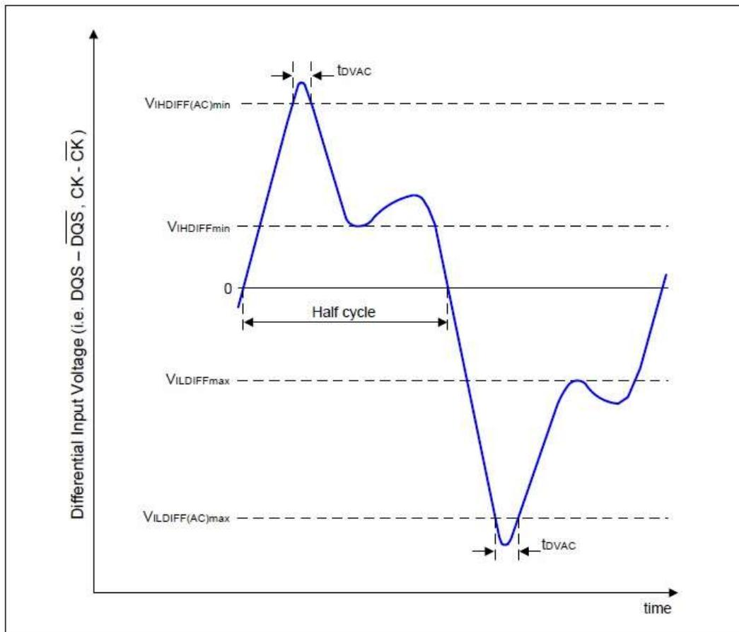
**Differential swing requirements for clock ( $\overline{CK}$  -  $\overline{CK}$ ) and strobe ( $\overline{DQS}$  -  $\overline{DQS}$ )**
