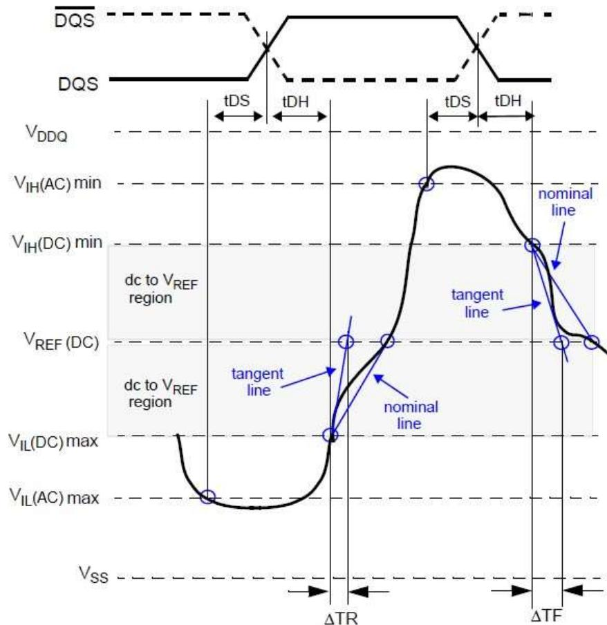
$$\text{Hold Slew Rate}_{\text{Rising Signal}} = \frac{\text{tangent line } [ V_{\text{REF}}(\text{DC}) - V_{\text{IL}}(\text{DC})_{\text{max}} ]}{\Delta \text{TR}}$$
