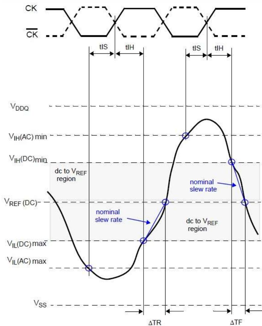
$$\begin{aligned} \text{Hold Slew Rate} &= \frac{V_{REF(DC)} - V_{IL(DC)} \text{ max}}{\Delta TR} \\ \text{Rising Signal} & \end{aligned}$$
