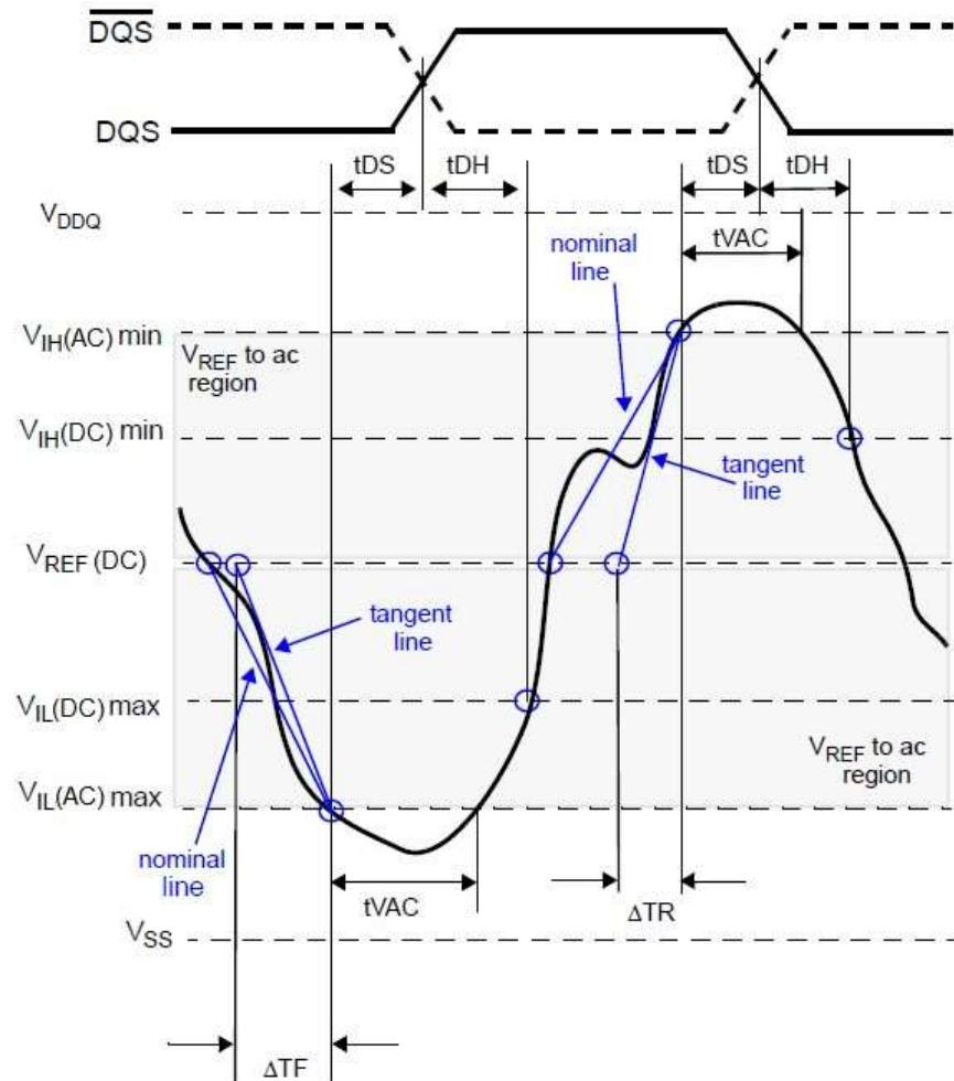
$$\text{Setup Slew Rate} = \frac{\text{tangent line}[ V_{REF(DC)} - V_{IL(AC)\max} ]}{\Delta TF}$$
