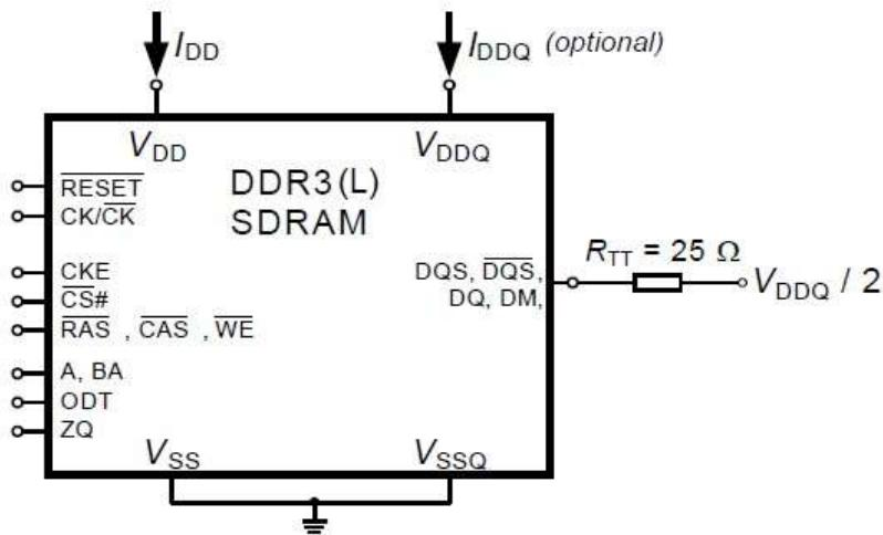
Note: DIMM level Output test load condition may be different from above.
