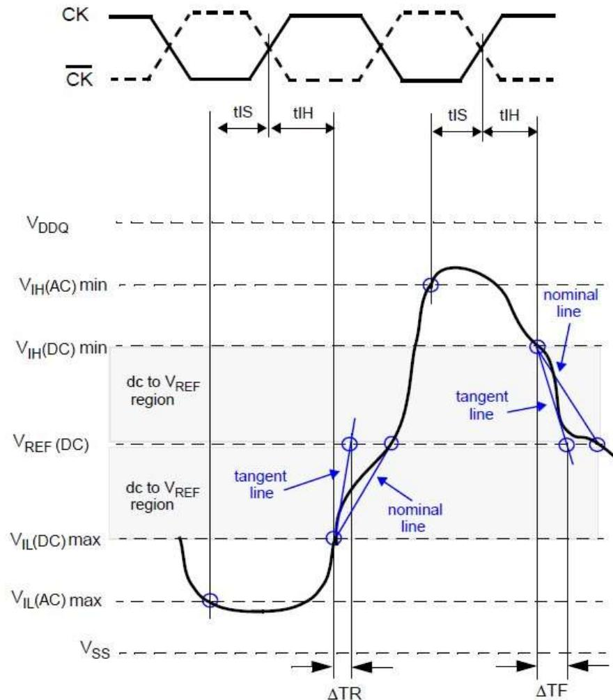
$$\text{Hold Slew Rate} = \frac{\text{tangent line } [ V_{REF}(DC) - V_{IL}(DC)\max ]}{\Delta TR}$$
