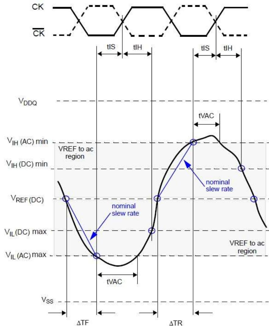
$$\text{Setup Slew Rate} = \frac{V_{REF}(DC) - V_{IL}(AC)\max}{\Delta T_F}$$
