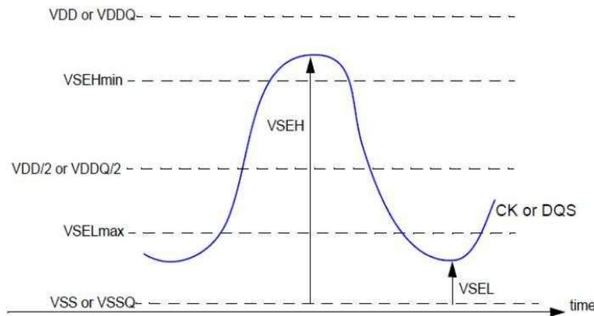
Note that, while ADD/CMD and DQ signal requirements are with respect to Vref, the single-ended components of differential signals have a requirement with respect to VDD / 2; this is nominally the same. The transition of single-ended signals through the ac-levels is used to measure setup time. For single-ended components of differential signals the requirement to reach VSELmax, VSEHmin has no bearing on timing, but adds a restriction on the common mode characteristics of these signals.
