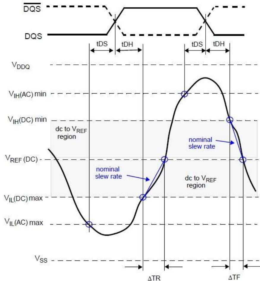
$$\text{Hold Slew Rate}_{\text{Rising Signal}} = \frac{V_{REF(DC)} - V_{IL(DC)\max}}{\Delta TR}$$
