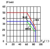
MAXIMUM FORWARD DC CURRENT VS, AMBIENT TEMPERATURE.
