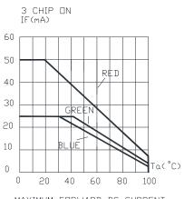
MAXIMUM FORWARD DC CURRENT VS, AMBIENT TEMPERATURE.
