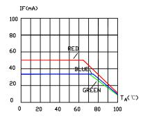
MAXIMUM FORWARD DC CURRENT VS, AMBIENT TEMPERATURE.
