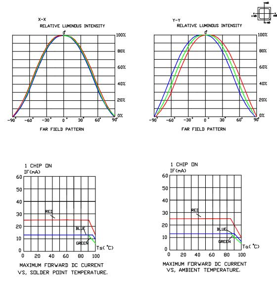
The graph shows the maximum allowable DC current for a LED die of each color.
