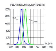
FIG.4 RELATIVE LUMINOUS INTENSITY VS. WAVELENGTH.
