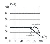
FIG.5 Blue MAXIMUM FORWARD DC CURRENT VS AMBIENT TEMPERATURE (Tjmex=110 $^{\circ}\mathrm{C})$
