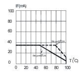
FIG.5 Green MAXIMUM FORWARD DC CURRENT VS AMBIENT TEMPERATURE (Tjmax=110 $^{\circ}$ C)
