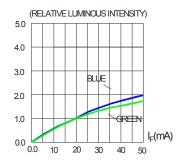
FIG.2 RELATIVE LUMINOUS INTENSITY VS. FORWARD CURRENT
