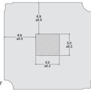
Tc measurement point: either the anode or cathode solder
