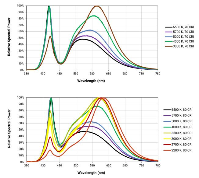
The following graphs are the result of a series of pulsed measurements at 1080 mA and  $T_{J}$  = 85 °C.
