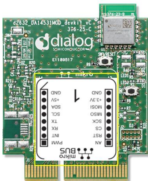
Figure 18: Example of mounting MikroBUS™ module
