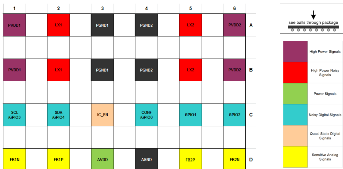
Figure 4: DA9220 Pinout Diagram (Top View)
