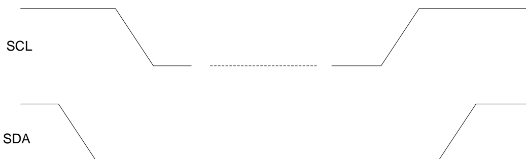
Figure 21: I 2 C START and STOP Condition Timing
