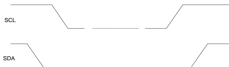
Figure 34: I 2 C START and STOP Conditions
