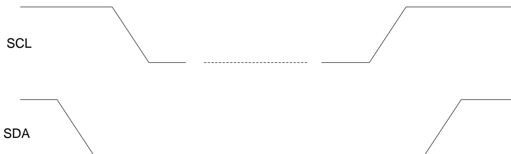
Figure 25: Timing of 2-WIRE START and STOP Condition
