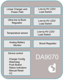
The device supports charge current up to 500 mA to speed up the charge cycle. The charge profile is programmable by resistors or in software, allowing either standalone operation or host control.
